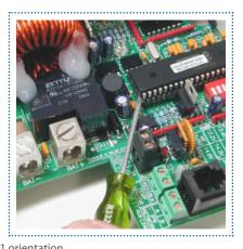
Reapply battery power. Confirm that the microprocessor operates by viewing the charge voltage 5. setting value (VCHG) as described in the SB3024 manual.
