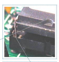
Confirm that each pin is properly placed into socket prior to pressing microprocessor into place.
