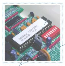
Place Microprocessor into socket with Pin 1 orientation where shown.
